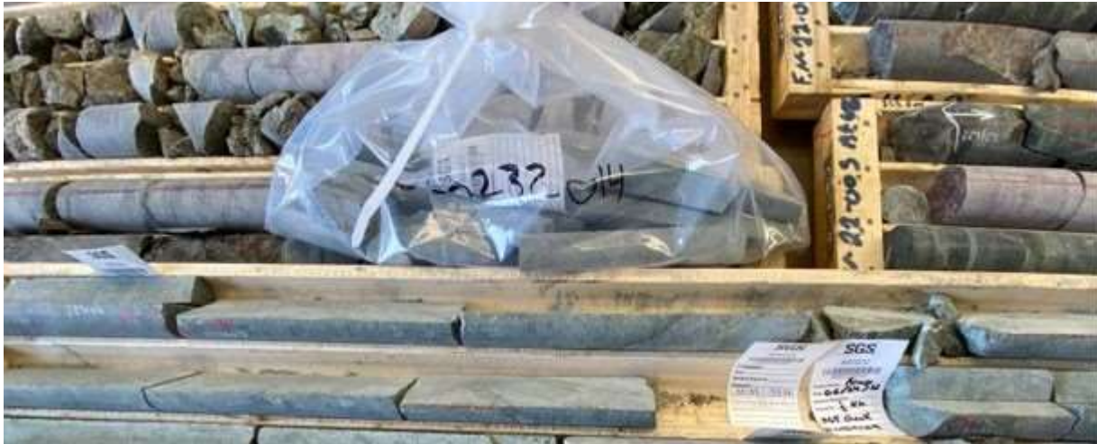
Figure 12-7: Example of quarter core check sample collected in 2022
