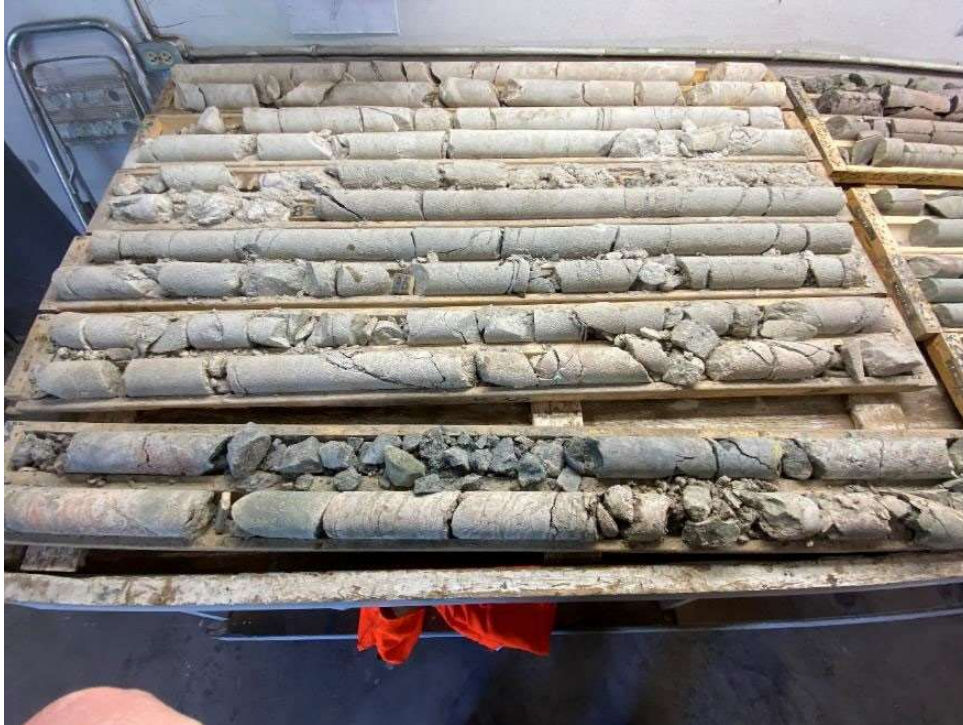
Figure 12-5: FN-22-005 drill core displaying limestone and sandstone units near top of hole
